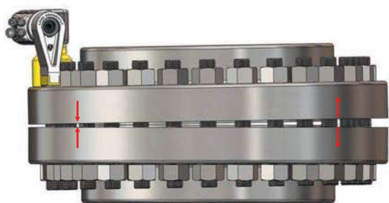
Uneven load using one tool
