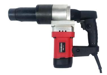
The PSW Series Shear Wrench is hand held, non-impacting electrically driven power tool is specifically designed to be used with Tension Control (TC) Bolts. The wrench enables bolts to ensure high axial tension and torque accuracy. The torsion shear bolts can be tightened by cutting off the spline. The operation is simple and convenient.
